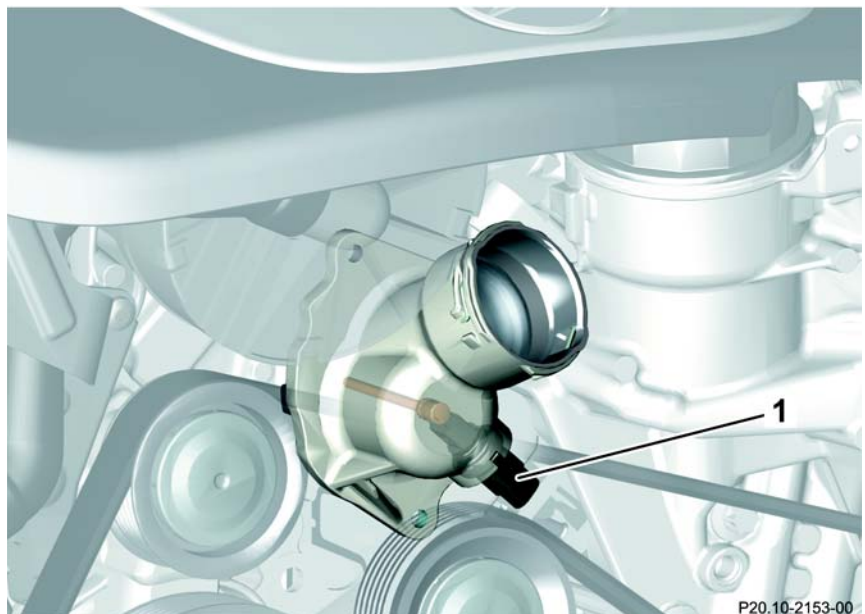
Triple-plate thermostat (Y110)
