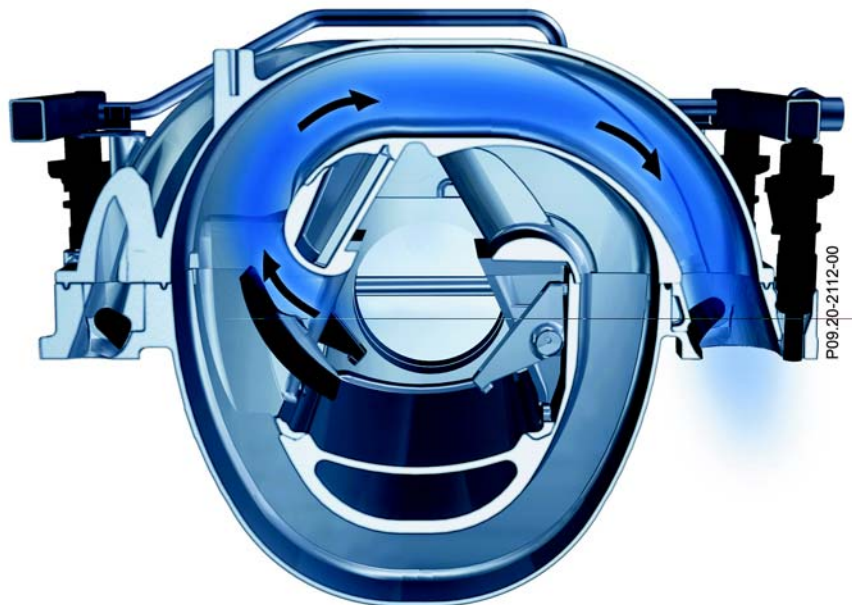
Routing flaps open, short intake channels
