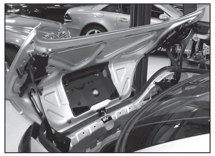
2 hydraulic cylinders open and close tubular frame. Design allows trunk lid to move rearward when opening and forward when closing
