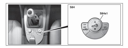
S84 Vario Roof/ATA switch groupS84s1 Vario Roof actuation switch
