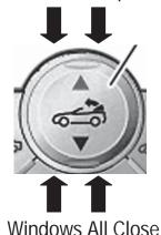
Door switches can't be used to close windows while Vario Roof is being operated
